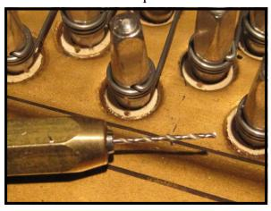
Sometimes if the tuning pin bushing is very tight, it may be necessary to drill a tiny hole through each bushing to allow the liquid to seep down to the pinblock. The drill in the photo to the left measures a mere .025", small enough to drill a hole in the thin wooden bushing surrounding each tuning pin. By drilling this hole, the liquid can better penetrate to where it's needed.
