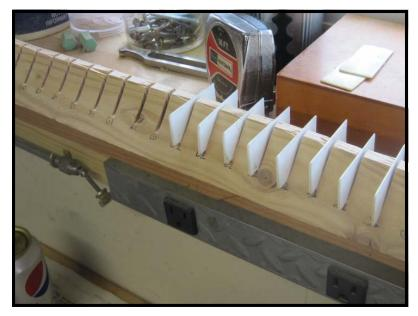
In situations where keytops are loose to the point where they are popping off unexpectedly, the only real solution is to remove them all, (usually both heads and tails) to reglue with proper methods that will ensure they stay put in the future. This is one potential aspect of the job which would add a great deal of shop time to the job.
