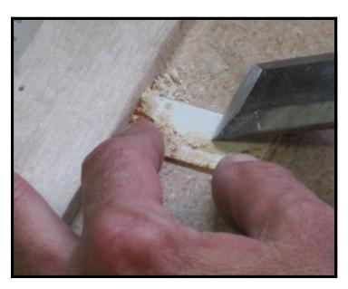
Next, any keytop which has been inexpertly glued to the keystick in the past must be removed and prepared properly. Many times an instrument will have ivories which are poorly glued, so that discolorations show through the translucent ivory. The only way to fix this problem is to remove the keytop and scrape the old adhesive off completely to start over with a proper job of gluing.
