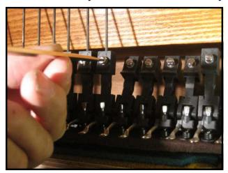
To access and remove the damper assemblies, the case will need to be disassembled to the extent that the action and keys may be drawn out of the piano. After removing the action from the piano, each damper will be taken out in order by loosening the set screw which holds the damper wire in place.
