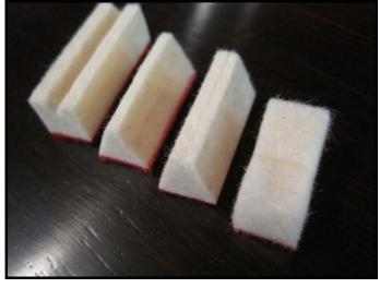
dampers (used for smaller steel treble strings). Obviously, a great deal of fine adjustment is necessary to make all these parts perform in unison with one another.
