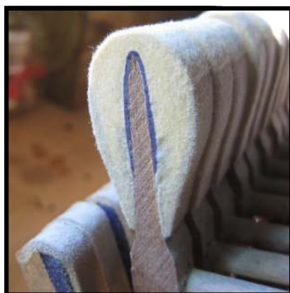
Worn hammer after filing
