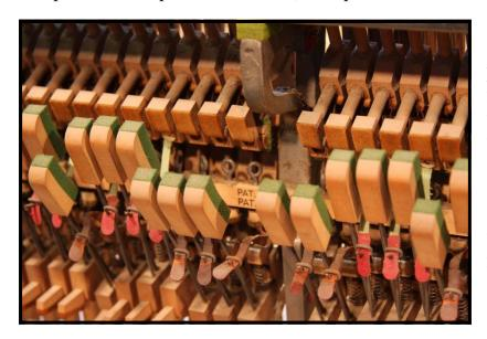
One example of parts which commonly needs to be replaced on a vintage upright piano is the bridle straps, shown in the photo to the left. These straps are essential for holding the bottom of the action up when it is removed from the piano for servicing.
